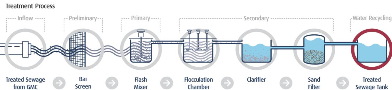
Note: Treated sewage is disinfected with hypochlorite to remove bacterial colony
